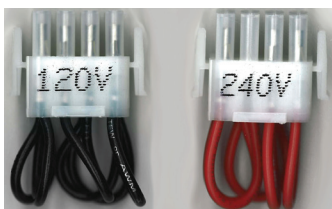
AC VOLTAGE SELECT PLUGS: (120 VAC or 240 VAC)
